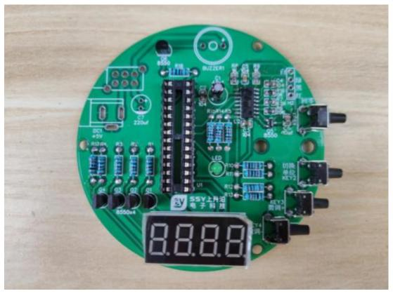
5: Finally, add welding other devices, the positive and negative of the buzzer need to be distinguished clearly; insert the single-chip microcomputer chip; the notch of the chip and the
